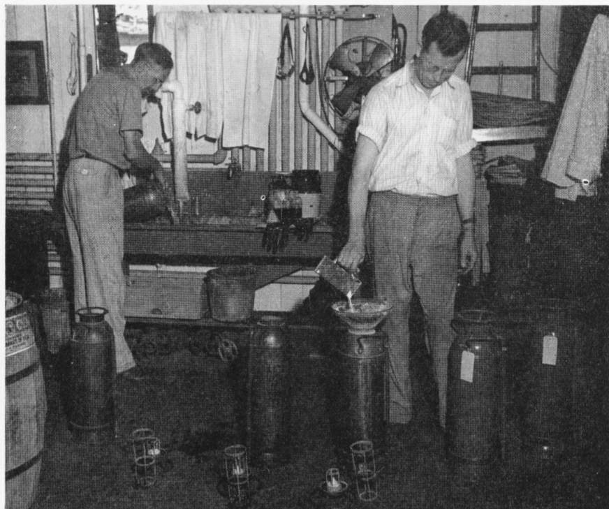
For highest efficiency the acid-soda type fire extinguishers must be serviced periodically. The contents of Scovill extinguishers are changed annually or following each use. Here J. G. Mathew pours out old ingredients, while Herman Hanson of the Fire House adds new soda.
